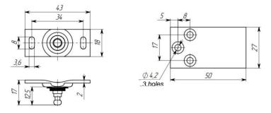
The pusher is located in the same casing as the lock, which allows not to mount a handle on the door. If necessary, positions of the lock and the pusher inside the casing can be interchanged; to do this, screw out the screw on the back side of the lock (may be hidden under the sticker) and remove the metal base of the lock.
