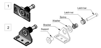
The latch is delivered in an assembled condition **1**, and is suitable for mounting on swing doors and drawers. For sliding doors of the rolling door cabinet type, it is advisable to use the position **2**. Mounting of the latch on the angular bracket is performed by the consumer in accordance with the above-presented diagram.
